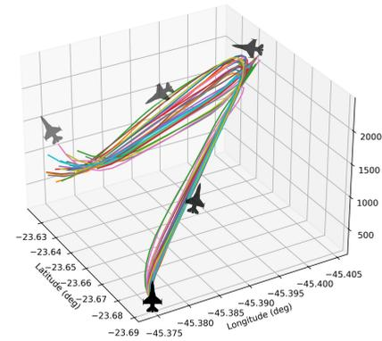
Figure 2. Adjusted flight data for the 30 flights of the pop-up attack maneuver executed by the human pilot.
