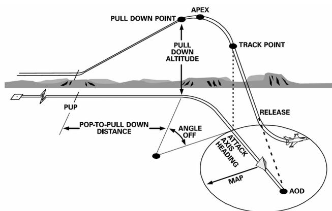
Figure 1. Flight profile for offset pop-up delivery. Source: Foo et al. (2009)
